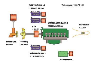
Example configuration: Pulling thruster and fixed pitch propeller in contra-rotating setup
