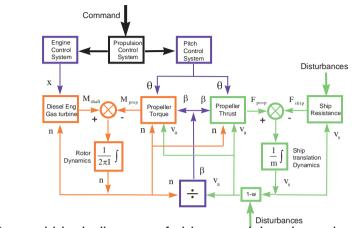
General block diagram of ship propulsion dynamics
